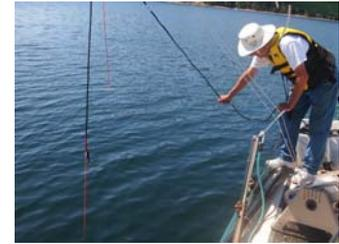
We use a YSI DO probe to check the dissolved oxygen in our 2 bays and Northern Hood Canal.
